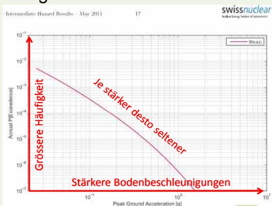
Fig. 2-1.9: Beznau, horizontal component, rock, surface, mean hazard, PGA.
